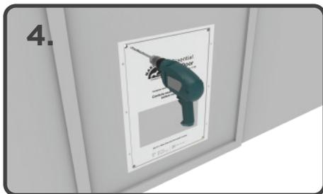
4. Drill a hole in each of the 4 inside corners with a minimum of 10mm (0.4") drill bit.
