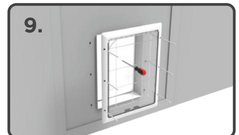
9. Screw into door from the inside. **WARNING: Over tightening of screws will cause damage.**
