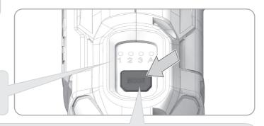
The "A" function is designed to give the user greater control in application and reduce damage to the fastener or work surface by automatically shutting the tool off after the tool senses the mechanism impacting for approximately one second.
