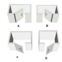
3.2 Depending on door opening direction, orientate the latch as required to align with the strike plate. (1)
