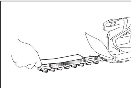
**NOTICE:** Do not wash the blades in water. Doing so may cause rust or damage to the tool.
