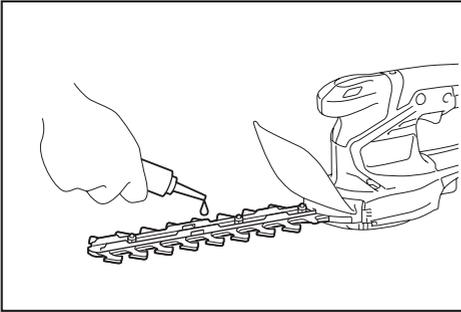
After operation, remove dust from both sides of the blades with a wired brush, wipe it off with a cloth and then apply low-viscosity oil (machine oil, or spray-type lubricating oil) to the blades.
