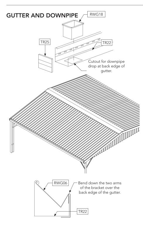
**1.** Attach end caps and join lengths of gutter **TR22**, to match the length of the edge beam by notching the roller edge of one to allow the other to slide into it.
