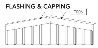
Fit barge capping **TR06** to the front and rear gables, fixing where there is a purlin beneath it using tek screws with neo washers.
