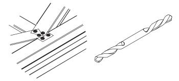
Absco sheds' frame sections are manufactured from light gauge steel, enabling for the notched ends or lengths of one frame section to be spread over the sides of another frame section, boxed frame section or H-section.
