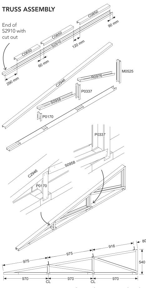
**1.** Take the bottom chord **S2910** and box-in the infill pieces at the distance specified. Fasten with wafer head tek screws.
