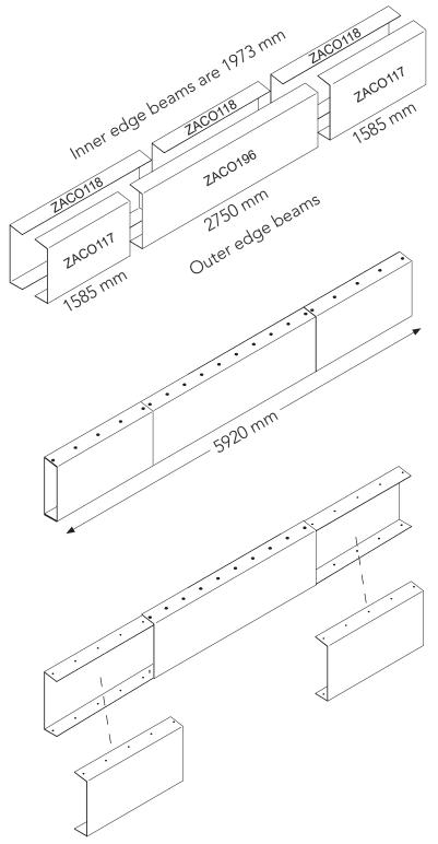
**1.** Arrange the six edge beam pieces as shown on the left.
