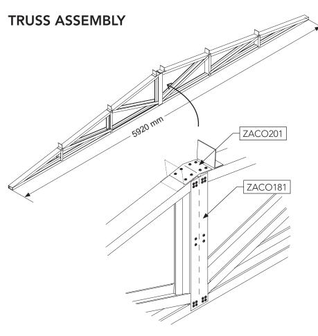
**5.** Butt two half truss assemblies together to make a single 5820mm wide truss.
