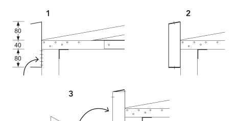
**1.** Place the posts on the foundation, use the dimensions shown to confirm correct placement.
