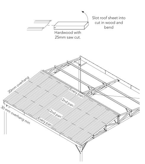
**Option.** On the ground, lay out the roof sheeting as if they were on the frame already. Using a piece of wood, as pictured, turn up the pans of each sheet at the end that's going to be at the ridge.
