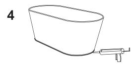
Apply wet area silicone sealant to the outer rim of the base of the bath, filling the 2-3mm gap. Allow 24 hours to cure before first use.
