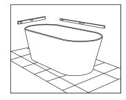
This bath is designed to be supported by the legs. Allow a 2-3mm clearance of the bath from the floor. Tilt the bath on its side (ensure the bath is adequately protected), and adjust the legs on the underside of the bath by loosening the nuts with a spanner in an anti-clockwise direction. Hand-twist the feet to the required height. Make minor adjustments to each leg until the bath is level in all directions. A non-level bath may not drain correctly. Re-tighten the nuts.
