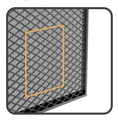
Tape and mark up the measurements needed to cut the opening.
