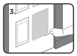
Cut out supplied template, line up with height (x) and trace on to door.
