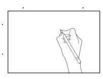
Position unit into the cutout hole, and mark the hole positions with a pencil. Put the unit aside.
