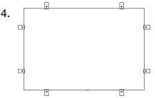
Carefully insert unit into cutout, make sure all holes are aligned with fixing clip holes. Fix with the screws provided ensuring the screws are inserted vertically so they engage with the backside of the fixing clip.
