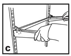
Attach assembly to Wallstrips by inserting lugs on Brackets into slots in Wallstrips and press down locking clips in Brackets.
