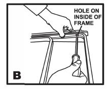
Using a Phillips Head screwdriver, fix the rear of the Frame to the Brackets by inserting and securing the self tapping screws. Insert them through the holes on the inside of the Frame and into the Brackets as shown in Diag B.
