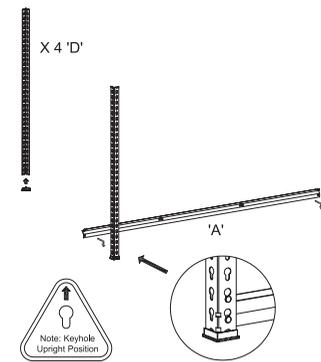
Place foot caps onto the bottom of the 4 legs 'D'. Note upright position. Place shelving bracket 'A' onto the legs 'D'. A rubber mallet can be used to lightly tap all brackets into the keyholes on the legs.
