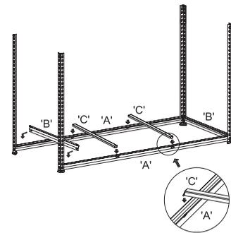
Use shelf bracket 'B' for the side brackets using the shelf bracket from Step 1 as a guide for height. Use same shelving brackets for opposing sides as shown in the diagram. Place brace 'C' as shown.
