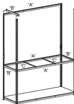
Place 1x MDF Shelf on the bottom brackets to minimise buckling. Fix brackets 'A' and 'B' at the very top of the leg uprights, then repeat with other brackets at your desired heights.
