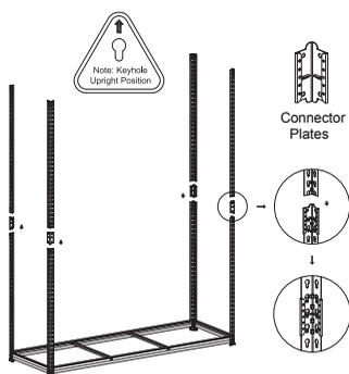
Join the upper legs to the lower legs with the connector plates.
