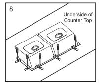
Lock the sink into the desired location. Be careful not to over tighten. Remove excess sealant.
