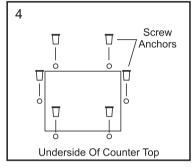
Insert each screw anchor into each drilled hole.
