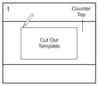
Place the cut out template into the desired sink location. Trace around the border of the template.
