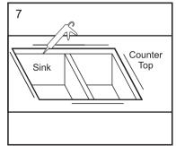
Apply suitable wet area sealant recommended for the stainless steel sink and counter top material.
