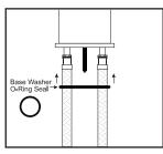
3. Place the base washer O-ring over the end of the hoses and insert into the base of the mixer.
