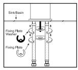
5. Position the fixing plate washer and fixing plate onto the bolt. The flexible hoses should be positioned towards the front of the sink/basin with the lever handle pointing towards the user. Fixing bolt positioned at the back.
