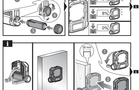
Use the magnets to mount the product on 22-gauge low carbon steel surface. Minimum thickness: 0.6 mm.
