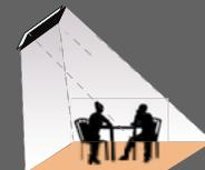
Angled mounting from the wall or ceiling is possible with the standard bracket, however the heating area is reduced
