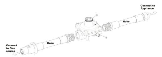
Note: The Regulator can't be repaired personal. If you have any question or problems, cut off the flow and call your distributors. No lubricant is necessary for assembling and the sealant can be used when connect the pipe. The sealant should be match with NG.
