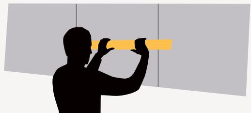
Note: Alter the thickness of silicone applied behind the different sizes of glass and polymer to obtain a flush finish across all materials. Pressing a straight edge against panels on the wall will assist with this.
