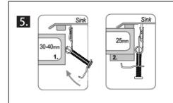
These anchor braces are designed for use with counter tops 30-40mm thick (1). If your counter top is thinner, insert wooden wedges between the counter top and the braces to secure them (2). After placing two at each corner of the sink, place the rest evenly spaced around the perimeter of the sink.
