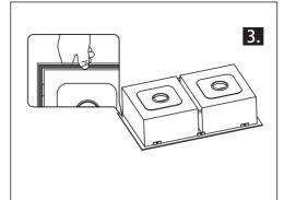
Adhere the bench seal around the under side of the edge of the sink, being careful to lay it smoothly (without ridges).
