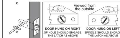
The spring loaded spindle will fit doors between 35mm and 65mm thickness. Cut the spindle to adjust the length to suit the door thickness.
