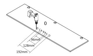
All doors have been pre-drilled to suit multiple handle hole spacings. If using the standard handle supplied, use the holes at 96mm hole centres marked (A) and complete the drilling process using the drill bit supplied.
