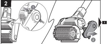
Press the latch to unlock the bracket. Remove the bracket.
