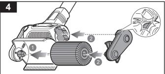
Install the replacement brush. Hold and press the bracket back in position until it clicks into place.
