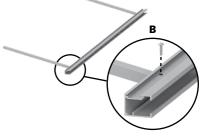
Insert the balusters into each end of the handrail (ensure the screw holes in the rail are facing up). Align the screw hole in each baluster with the screw hole in the handrail, then fasten each baluster to the rail using 12 mm pan head self-drilling screws.
