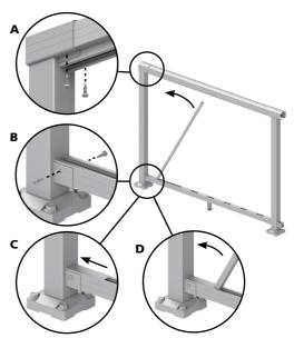
A: Install the base rail support into the bottom channel of the base rail.
