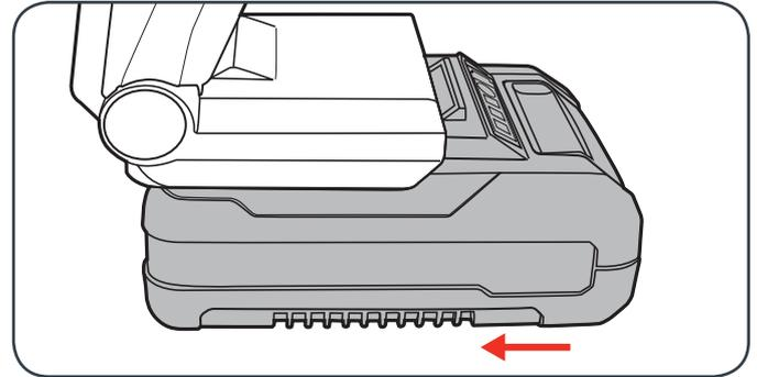
2 To remove, press and hold the battery release tab and pull the battery away from light.
