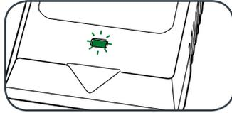
3 With the battery sitting on a flat surface, align the raised ribs on the battery with the recess in the charger and slide onto the battery ensuring a firm connection.
