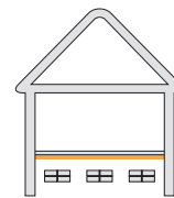
Sub-floor solid perimeter
