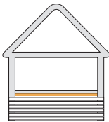
Sub-floor with timber battens
