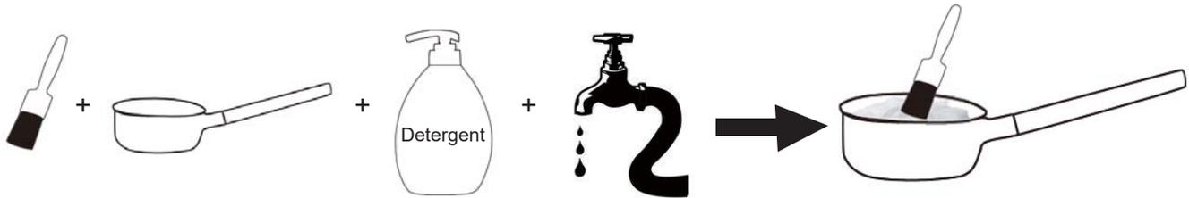
Make sure the control knob on the heater is off and the gas valve on the cylinder is off before mixing the soapy solution.
