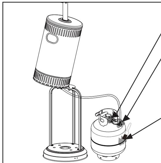
Soap bubbles will appear if there is a gas leak. In case of a leak, turn off the gas supply. Tighten any leaking fittings, then turn the gas supply on and re-check.
