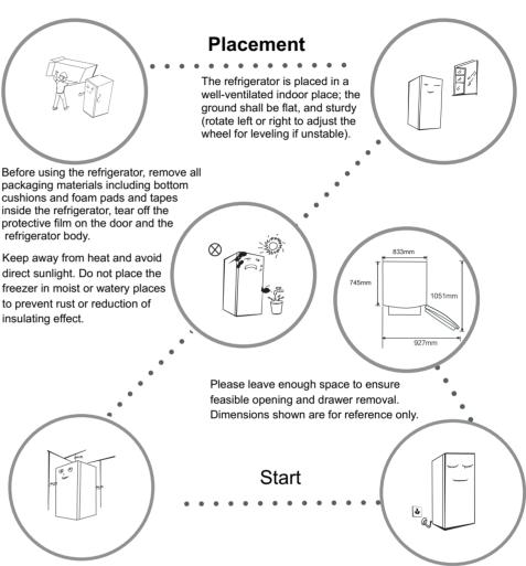
The top space of the refrigerator shall be greater than 30cm, and the distances from both sides and backside shall be more than 10 cm to facilitate the opening and closing and heat dissipation. Wipe the refrigerator inside and outside with warm moist rag (add a small amount of detergent in the warm water and wipe clean finally with clean water).
