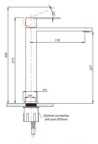
Unless specified, dimensions are in millimetres (mm).
