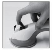
Lift up (unlock) the blue tabs on the support bar.
