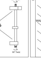
Twist and lock the mounting brackets into correct installation position.
