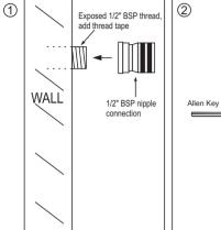
Apply thread tape before installing
