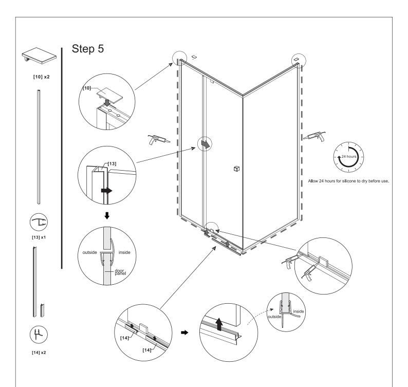
Note: Make sure the door seal is installed according to the instructions and the door is opened outward. If the door seal is installed in the opposite direction, the door is opened inward, there may be water leakage.
