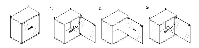
If required, adjust the Door to get an equal gap.
