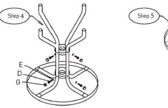
When all the bolts are in position, tightly secure using Allen Key (F). Then insert the bolt caps(G).
