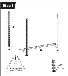
Add Foot End Caps to bottom of Legs 'C'. Fix Brackets 'A' to the bottom of Legs 'C' as shown. A rubber mallet can be used to lightly tap all brackets into the keyholes of the legs. Allow one keyhole free between the foot end cap and the shelving bracket.
