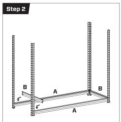
Fix Brackets 'B' to the bottom of Legs 'C' as shown. A rubber mallet can be used to lightly tap all brackets into the keyholes of the legs. Allow one keyhole free between the foot end cap and the shelving bracket.
