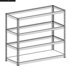
Fix remaining Brackets 'A' and Brackets 'B' to desired shelf height. As before, a rubber mallet can be used to lightly tap all brackets into the keyholes of the legs.
