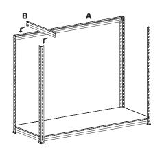
Fix Brackets 'A' to the top of Legs 'C' as shown followed by Brackets 'B'. A rubber mallet can be used to lightly tap all brackets into the keyholes of the legs.
