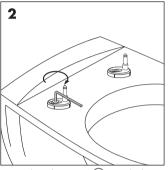
Semi-tighten the screws © in a clockwise Clip on the toilet seat ©. direction. Do not fully tighten, as the position of the hinges ® may need to be adjusted.
