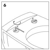
Fully tighten the screws  $\bigcirc$  in a clockwise direction.
