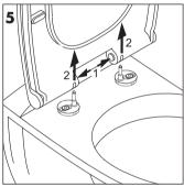
Remove the seat (E) by pressing the release buttons, then lifting it upwards.
