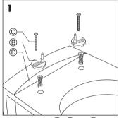
Insert components (B), (C) and (D) into the pan.
