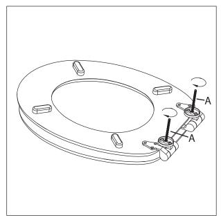
Screw the threaded rods (A) into the hinges.
