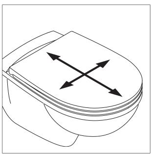
3. Place the seat – with the threaded rods (A) attached – onto the pan and align. Carefully remove the seat ensuring that the position of the hinges are not altered. Tighten the hinges.
