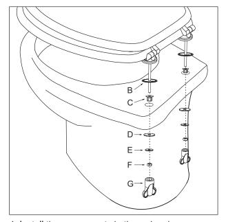
4. Install the components in the order shown above, and hand-tighten the wingnuts (G) to secure the seat to the pan.
