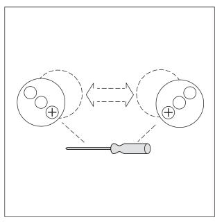
2. Slightly loosen the hinges with a screwdriver and adjust the width to suit the toilet pan holes.
