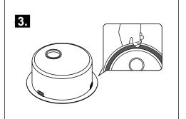
Adhere the rubber bench seal around the under side of the edge of the sink, being careful to lay it smoothly (without ridges).
