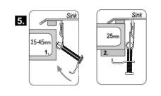
These anchor braces are designed for use with counter tops 35-45mm thick (1). If your counter top is thinner, insert wooden wedges between the counter top and the braces so as to secure them (2). After placing two at each corner of the sink, place the rest evenly spaced around the perimeter of the sink.
