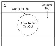
NOTE: BEFORE CUTTING, DOUBLE CHECK THE MEASUREMENTS OF YOUR TRACED LINE IS ACCURATE TO YOUR BOWL DIMENSIONS.
