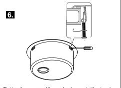
Tighten the screws of the anchor braces (with a hand screwdriver), to secure the sink in place.
