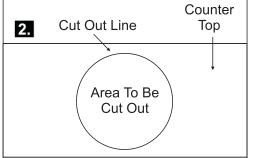
NOTE: BEFORE CUTTING, DOUBLE CHECK THE MEASUREMENTS OF YOUR TRACED LINE IS ACCURATE TO YOUR BOWL DIMENSIONS.
