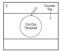
Place the cut out template into the desired sink location. Trace around the border of the template.
