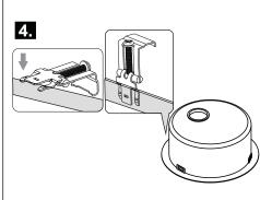
Place the anchor braces vertically and pull them up to lock into their horizontal position.
