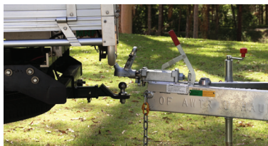
Photo 1 - Reverse vehicle close to trailer
