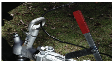
Photo 3 - Thread lead through coupling handle
