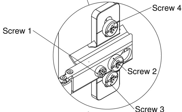
To adjust the gap between cabinet top and door, loosen screw 3 and 4 of top and bottom hinge by turning screws in anticlockwise direction. Adjust the gap between cabinet top and top of the door. Once adjusted, tighten the screw 3 and 4 by turning in clockwise direction.
