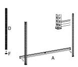
Add Rubber Feet (Part F) to bottom of 4 Angle Posts (Part D). Note upright position. Slot Long Beams (Part A) to the bottom of the Angle Posts (Part D) as shown into keyholes.
