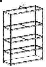
Apply remaining Beams as above to desired height. Ensure that Braces (Part C) are fixed to all shelves
