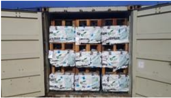
Examples of void fill (timber packing) in containers to stabilise the load
