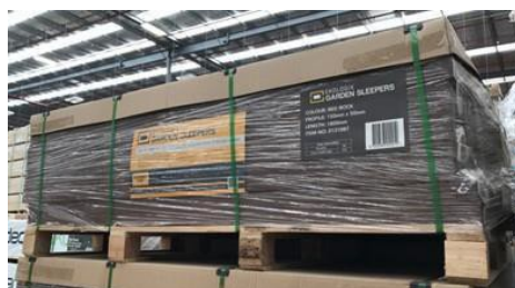
Example of a well packed and labelled timber pack
