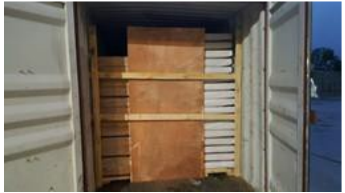
Examples of void fill (timber packing) in containers to stabilise the load
