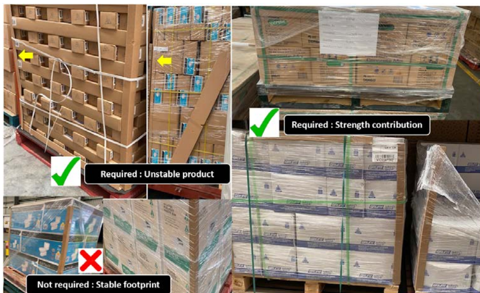
Examples of products having corner posts usage and some which do not require.
