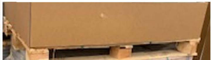
Cardboard sleeve or collar on lower portion of pallet can help reduce/dampen shock
