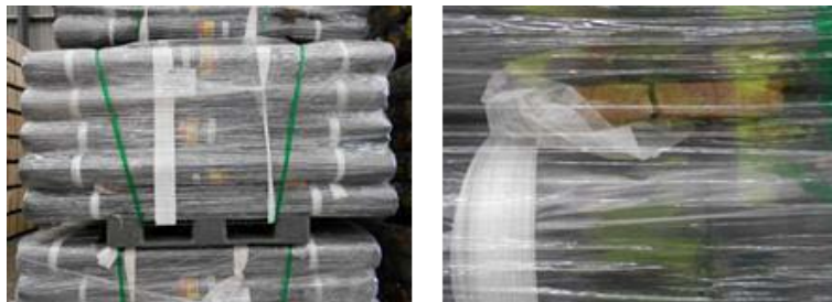
Example of oversized product on purpose made pallets, supported with strapping.
