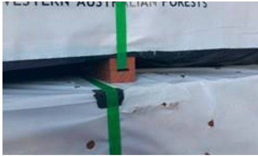
Example of a timber pallet with a bearer that is too thin and incorrect labelling standard
