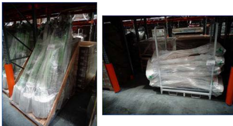
Example of support skids in use. Storing products in this manner saves on rack space and allows for efficient container unload and movement through the Distribution Centre.
