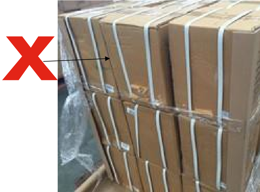
Example of damage to cartons when sticky tape was used to secure corner posts
