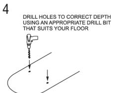
DRILL HOLES USING AN APPROPRIATE DRILL BIT. APPLY WET AREAS SILICONE INTO THE HOLES & TO THE BASE OF THE FLOOR BRACKET TO HELP KEEP THE FLOOR WATERPROOF. INSTALL THE FLOOR BRACKETS INTO POSITION. DON'T INSTALL SS SCREWS AT THIS POINT.
