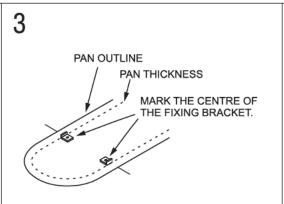
REMOVE THE PAN & MEASURE THE DESIRED SCREW FIXING POINTS. REMEMBER TO ALLOW FOR THE PAN THICKNESS. A 1-10MM GAP BETWEEN THE PAN & FIXING BRACKET IS ACCEPTABLE.
