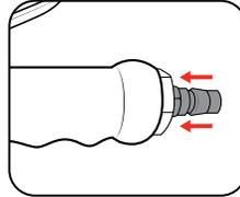
2. Screw in Nitto Style Fitting to the air inlet of the Air Angle Grinder.
