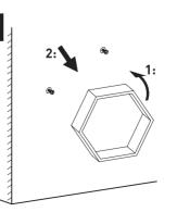
Please perforate holes on the wall based on actual distance between holes for wall mounting.
