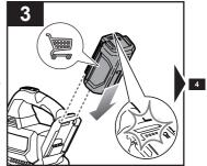
Insert the battery pack into the battery port until it clicks into place.
