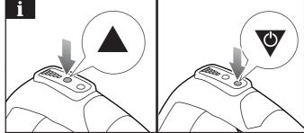
**NOTE:** Press the speed up button to increase the speed of the product. Press and hold the power button to decrease the speed of the product.
