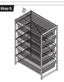
**Please note:** For stability and safety, fix the unit to a wall with the provided brackets. Place the brackets over the rear frame legs and attach to your wall. Necessary fixings for these brackets can be found at your local hardware store.
