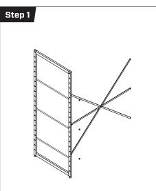
Align the cross-bracing to the 3 holes on the back of the frame and fix with the provided screws. Please note: Adjustable feet on the frame should be positioned at the bottom.
