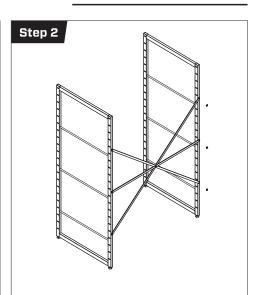
Repeat step 1 for the remaining frame. Please note: Adjustable feet on the frame should be positioned at the bottom.
