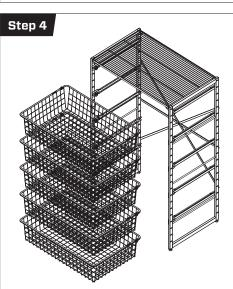
Attach the drawer runners at your desired heights by pressing them into the slots on the frame.
