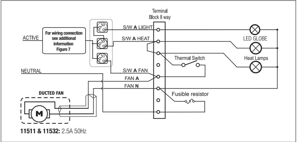
Fig. 5: Wiring diagram for model 11511 & 11532
