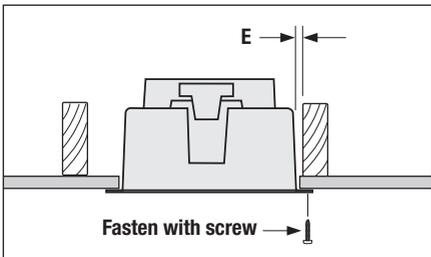
Fig. 3: Joist clearances
