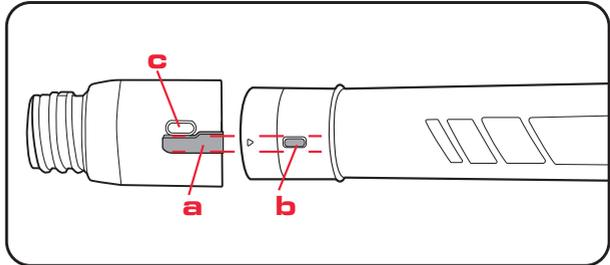
2. Rotate the adaptor to lock the raised tab (b) in opening (c).
