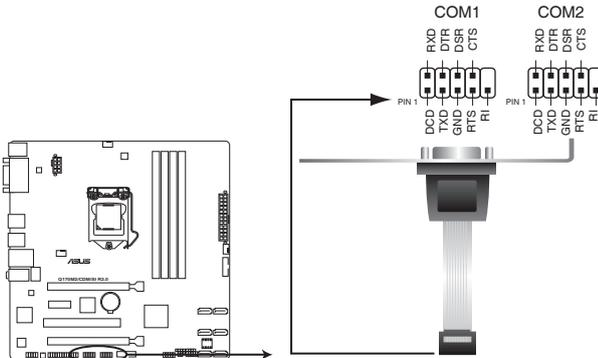
**Q170M2/CDM/SI R2.0 Serial port (COM) connectors**
