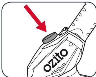
2. Tilt the cutter head to the desired angle.
