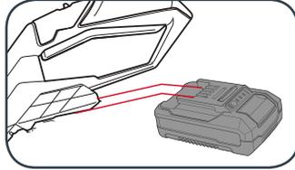
2. To remove, press and hold the battery release tab and then slide out.
