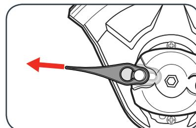
3. To remove the blade push the blade towards the centre of the spindle and then slide off.
