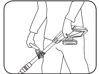
3. To turn on squeeze the on/off trigger whilst holding the lock-off button down.
