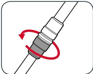
2. Extend to the desired height and then retighten the shaft adjustment collar to secure in place.
