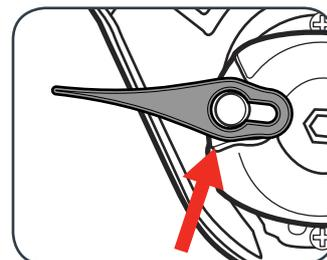
2. Pull the blade outwards so that the small hole is fitted into the mount.
