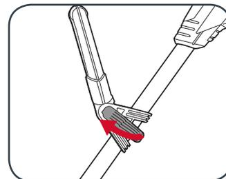
2. Rotate the handle into the desired position and then lock in place with the lever.
