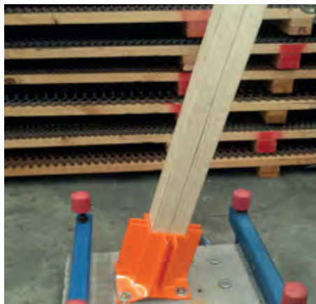
Safety base tested to 3160 Newtons without failure
