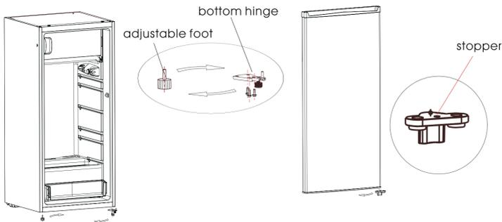
5. Install the door to the bottom hinge, install the upper hinge, upper hinge cover and hole cover on the other side
